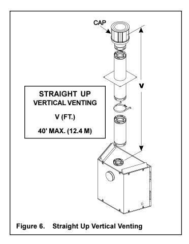
**NOTE:** On vertical venting configurations where the vertical component is over 10 feet, you may want to install the vertical baffle (VERT-BAF) (see Figure 7).
